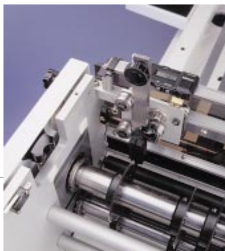
Above - The auto-feed Multiscore maintains optimum feed speed. Shown with four clamp arrangement for simultaneous dual axis scoring.
